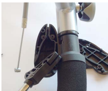
11. Put the new wire into the Brake Inner Part. Put the wire into the rear profile as shown in picture 7, 6, 5, 4, 3, 2, 1.
