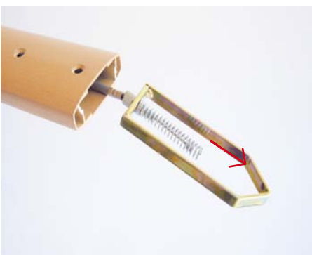
4. Remove the spring from the end of the wire.
