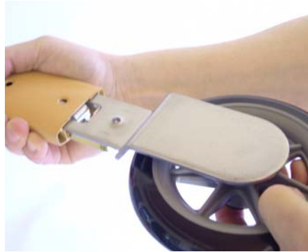
2. Pull out the rear wheel and the brake mechanism.
