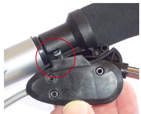
12. Push in the peg into the hole in the handle tube and screw the cover in place. Replace all as in picture 7, 6, 5, 4, 3, 2, 1.
