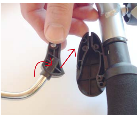
10. If the Brake Inner Part is damaged it can also be exchanged. Turn it a quarter of a turn and pull it off the bow.
