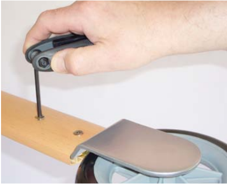
1. Unscrew the two Allen screws at the bottom end of the rear profile.
