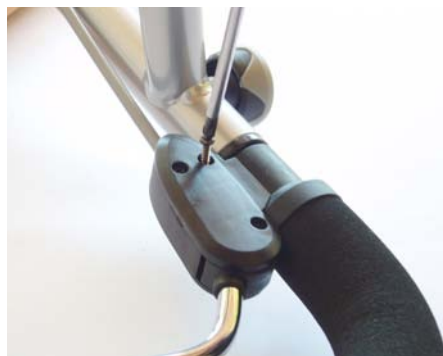
8. Unscrew the three parker screws from the brake housing.
