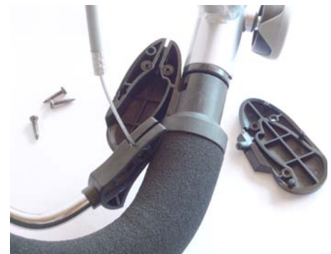
9. Loosen the wire from the Brake Inner Part at the brake bow. The wire can now be exchanged for a new wire.
